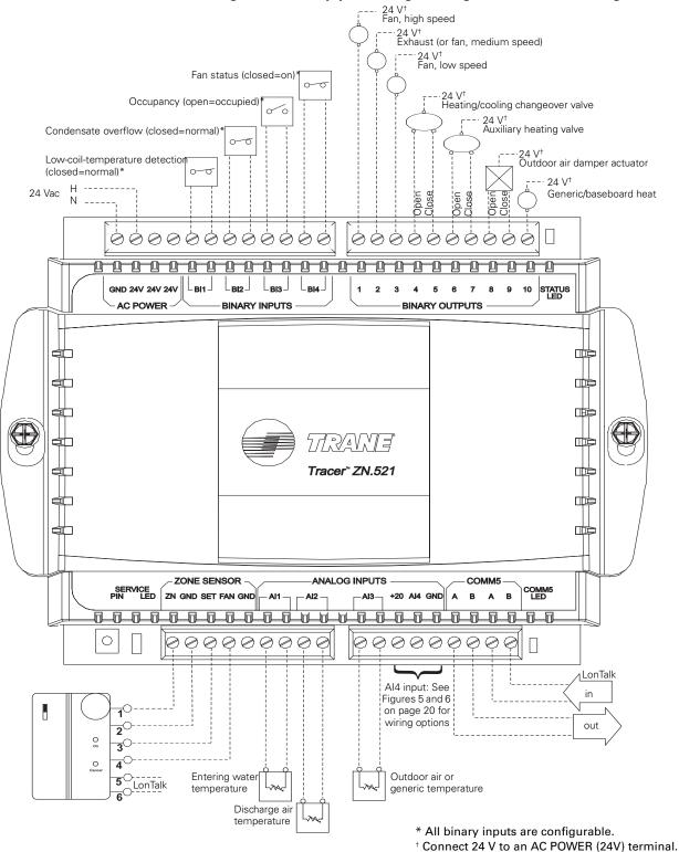
Figure 11. Four-pipe heating/cooling unit with auto changeover
